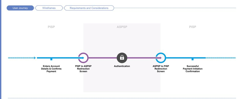
PSU Authentication with the ASPSP using browser based redirection for a PIS request.
