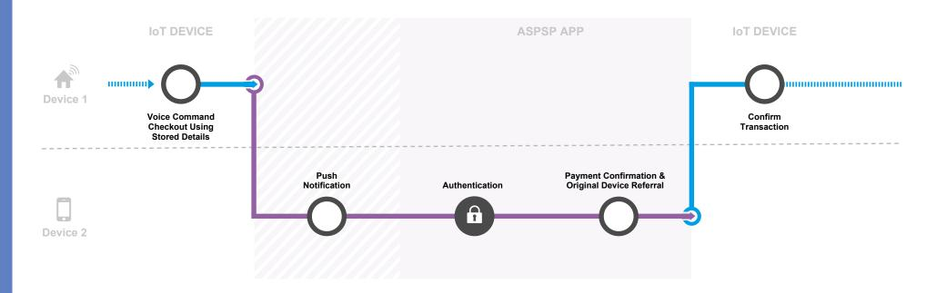
A decoupled authentication flow where the TPP (AISP/PISP/CBPII) provides the ASPSP a stored PSU identifier, generated by the ASPSP from a previous PSU transaction. This is used by the ASPSP to notify the PSU such that the PSU can authenticate using the ASPSP app on a separate device.
