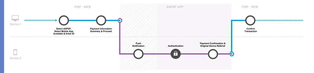
A decoupled authentication flow where the PSU provides a static identifier to the TPP (AISP/PISP/CBPII) which is used by the ASPSP to notify the PSU, such that the PSU can authenticate using the ASPSP app on a separate device.
